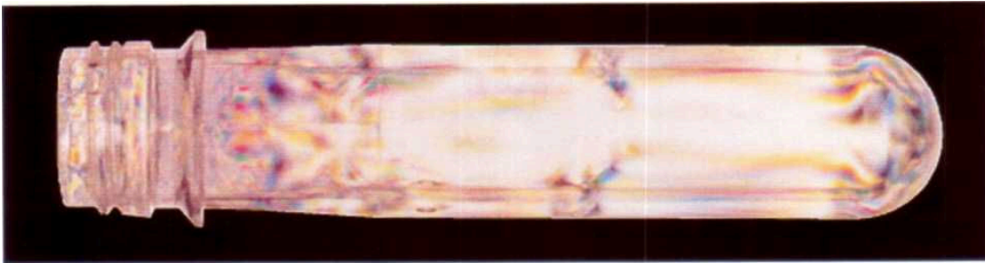
PET preform viewed under polarised light with preform held at 45° to the polarising axis
