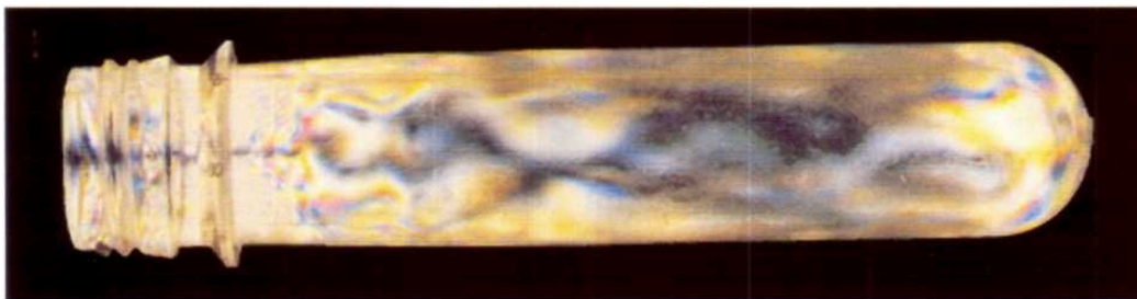
PET preform viewed under polarised light with preform held parallel to the polarising axis
