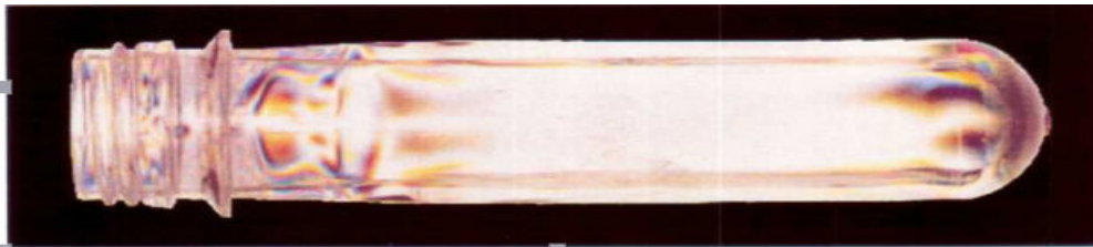
PET preform viewed under polarised light with preform held at 45° to the polarising axis
