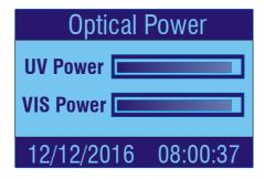
The "UV Power" level bar indicates the power of the UV LED. The "VIS Power" level bar indicates the power of the VIS LED.
