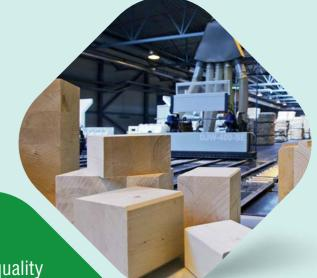
Perfect quality gluing using modern equipment HFC-press Kallesoe (Denmark), which provides glue line heating at molecular level.
