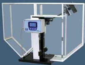
Impact Testing machine 20 J
