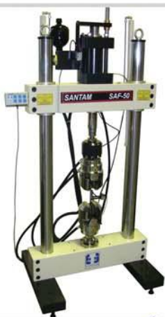
Axial Fatigue Testing Machine 20 kN
