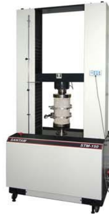
Universal Testing Machine 150 kN
