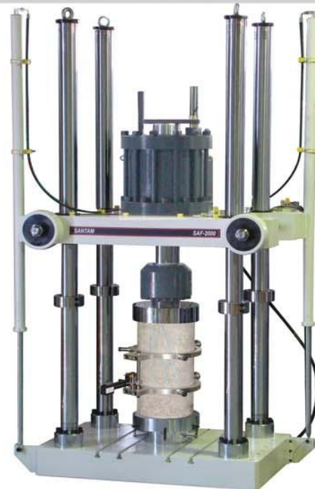
Universal Testing Machine 150 kN
