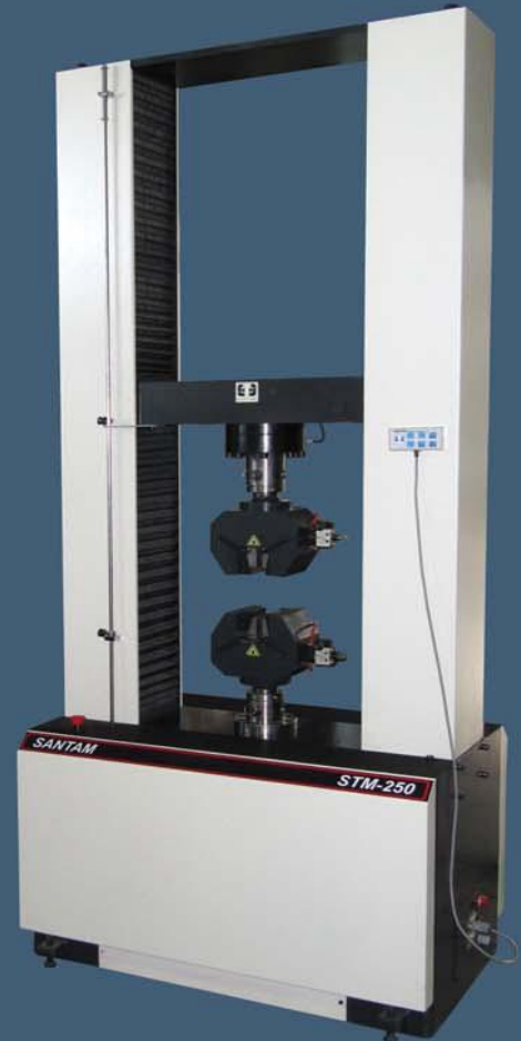
Universal Testing Machine 250 kN
