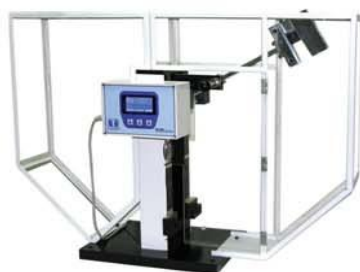
Impact Testing Machine 20 J
