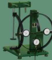
SDB-30 Curved Beam's Bending
