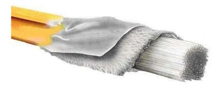
These pultruded bars can be cut into requested lengths. The bars are then drilled on the sides to accept the crossbars. The drilled bars are spaced. The final step is to seal the entire crossbars and holes with corrosion resistant epoxy resin.
