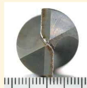
ABREX 500 Powder High Speed Steel 4.7m/min 0.25mm/rev Plated Through Hole: 53
