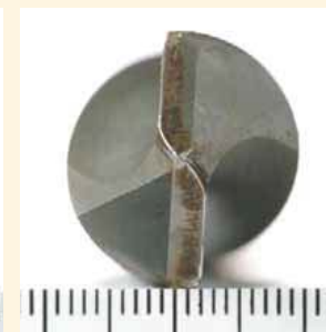
ABREX 400 Powder High Speed Steel 4.7m/min 0.25mm/rev Plated Through Hole: 136
